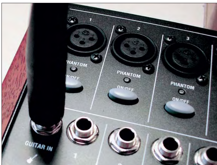
Below: The phantom power microphone inputs on the D3200 provide the electrical charge that is needed for condenser microphones
