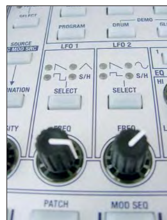
Above: Add movement with the two onboard low-frequency oscillators
