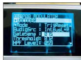
Above: The onboard vocoder is 16-band so it's capable of recreating most of the classic vocoder effects we all know and love
